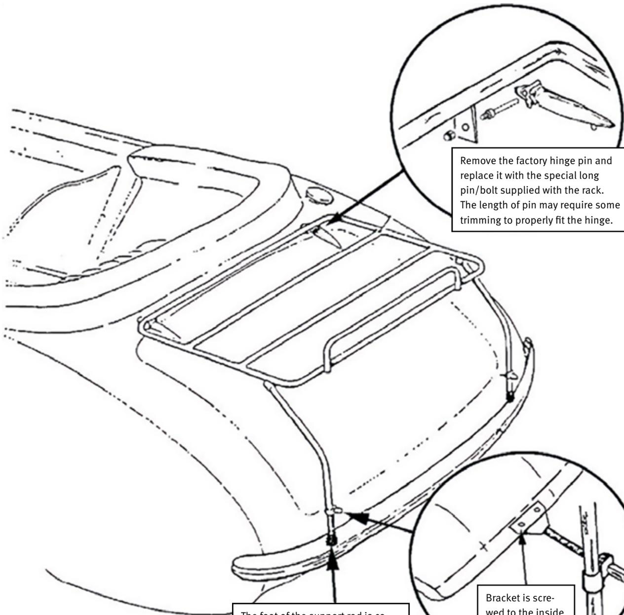
Remove the factory hinge pin and replace it with the special long pin/bolt supplied with the rack. The length of pin may require some trimming to properly fit the hinge.
