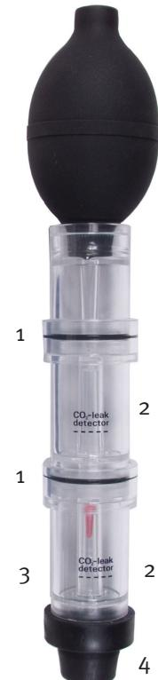
Use only clean CO<sub>2</sub> gas (exhaled air) for the sensitivity test and normal fresh air to regenerate the fluid. Never use exhaust gas directly or smoke from matches, candles light, tobacco etc. . Such gas contains residues which will contaminate the fluid and reduce the sensitivity.
