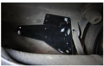
7. Ensure the bracket remains snugly fitted against the axle strap bracket and surfaces A + B before drilling the remaining holes. bracket before securing with the smaller washer and nyloc nut. It is preferable when mounting the boot floor bracket to have an assistant to help with the tightening of the fixings. NB Remember to replace the plain nuts with nylocs for final assembly. Tightening of the nuts will result in a dishing of the large washers. Torque to 20 ft/lbs. (See Images below)
