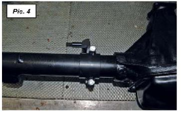
4.2 Fit the axle bracket so the large section is below the axle, pointing forward, with the pins pointing outwards. Fit the smaller section of the bracket, hardware and secure leaving it loose enough to allow for final positioning.
