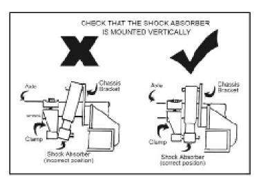
6.1 The shock absorbers should be vertical when viewed from the rear of the car (see Pic.8) and lean forward viewed from the side (see Pic.9). Adjust the location of the axle brackets to achieve this position. The split between the two sections should be roughly horizontal (bear in mind if the car is horizontal or raised at the rear) and so that the lower edge of the bracket, near the shock absorber pin, is not lower than the rear leaf spring (see Pic.10).
