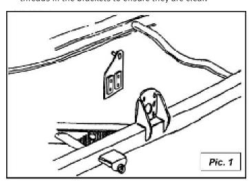
3.2 This conversion requires the drilling of two additional holes in the lower section of the chassis brackets. Using the existing lever arm damper mounting holes, install the new shock absorber brackets on the inside of the chassis brackets, ensuring the pins point to the centre of the car, do not fully tighten (see Pie.2).
