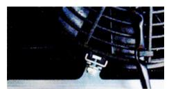
4. Loosely assemble the 4 square bolt kits and slide each of the heads into the slots with the square plate between the fan and the bracket with the washer and nylock nut on the outside. Making sure the fan is pressed securely against the radiator tighten each of the 4 nuts to secure the radiator in place. Refit the shroud and refit assembly to car.
